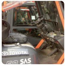
Instrument display and hydraulic levers in working order
