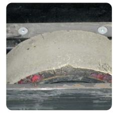
► Thermal deformation of tread or tyre walls
