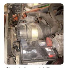
Starter battery and air filter in working order
