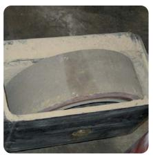
Tyres/rollers sit snugly on wheel rims and are within wear parameters according to local accident prevention regulations
