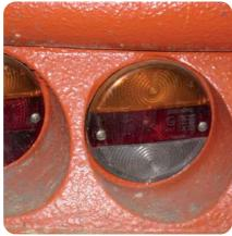
Plastic casing, mount, and glass all undamaged
