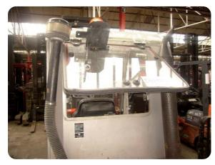
All cabin functions usable (front and rear windscreen wipers, heating and ventilation system, cabin lighting, roof hatch, mirrors, rear windscreen heater, radio, window opening mechanism)
