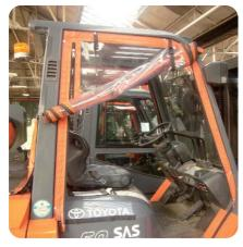
▶ Doors, front and rear parts all present, not deformed and in working order
