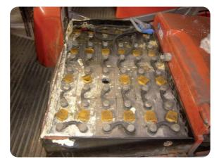
▶ Damaged battery-missing plugs
