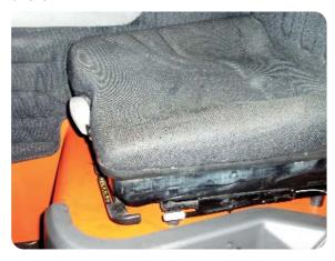
▶ Acceptable seat condition, worn but not torn, no holes or cuts, seat complete
