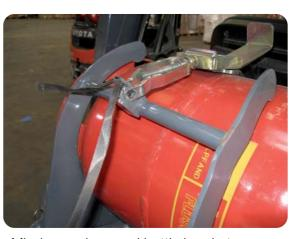
▶ Missing or damaged bottle brackets
