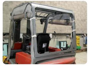
▶ Make sure that the overhead guard is in perfect condition: no bend, no dents of the overhead guard pillars or roof
