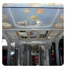
▶ Cabin spars or parts (roof, doors, front windscreen, rear windscreen) incomplete and/or deformed
