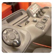
▶ Plastic dashboard without chunking, cracks or broken sec
