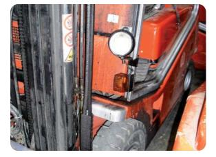
▶ Hydraulic connections in working order and without any major leaks
